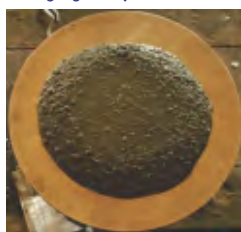
M-Sand mortar flow at 85% flow (no segregation) for 1:6 mortar
