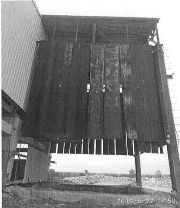
Water sprinkling & rubber Curtains @ Limestone Hopper
